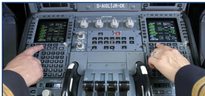
Flight Management System & Multifunction Control Display Unit
